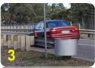
Guard Rails<sup>1</sup> are engineered to absorb the kinetic energy of an impacting vehicle. This is accomplished by deforming (flattening) the guardrail. End terminals are designed to reduce the problems associated with impacting vehicles, such as spearing, vaulting and rollover. Images 1 and 3 are two designs to absorb the impact. Image 2 is a slightly curved end of a straight guardrail (fishtail model) – 2a shows the knife edge end close up from image 2. All photos taken in Australia.
